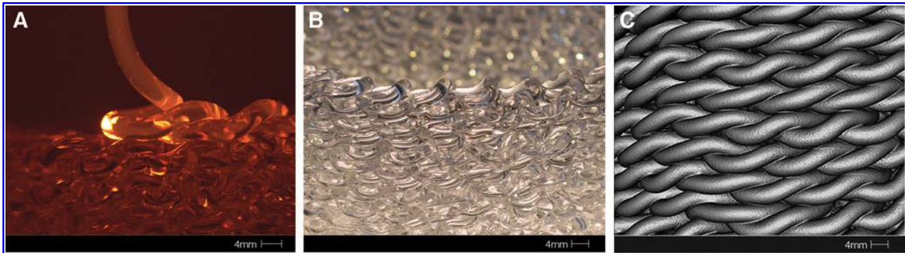
FIG. 6. Falling fluid deposition: (A) deposition process (Image Credit: Steven Keating), (B) photographic detail of the printed object, and (C) a higher magnification 3D reconstruction from micro-computed tomography data.
