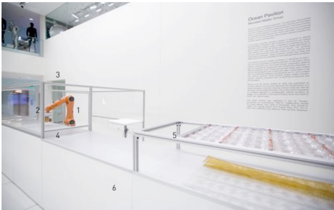
Figure 3: Perspective view of the manufacturing platform installed at the MIT Media Lab composed of (1) a positioning robotic arm (Kuka KR AGILUS robotic arm, model KR 10 R1100); (2) a customized multi-barrel extrusion head for water-based materials; (3) a security envelop for operation of the robotic assembly; (4) a 1m-wide and 5m-long deposition bed; (5) a computer-controlled evaporation system composed of 100 fans; and (6) a 9m-long workspace and storage cabinet.
