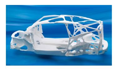
**Figure 2.** The Mercedes-Benz Bionic Car Project. Image illustrating the Soft-Kill Optimization (SKO) method implemented on a solid block of material to form-find the automobile optimal shape. The fabricated material is characterized by homogenous properties. Source: <a href="http://www.carbodydesign.com">http://www.carbodydesign.com</a>
