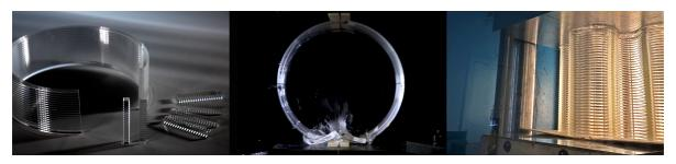
Figure 5: Laboratory tests on the glass products: rectangular bar samples for small-scale tests prepared from the cylindrical prints (left), full-scale bending test along the corrugation of the printed layers (middle), and full-scale compression test on a component used for one of the glass columns (right)
