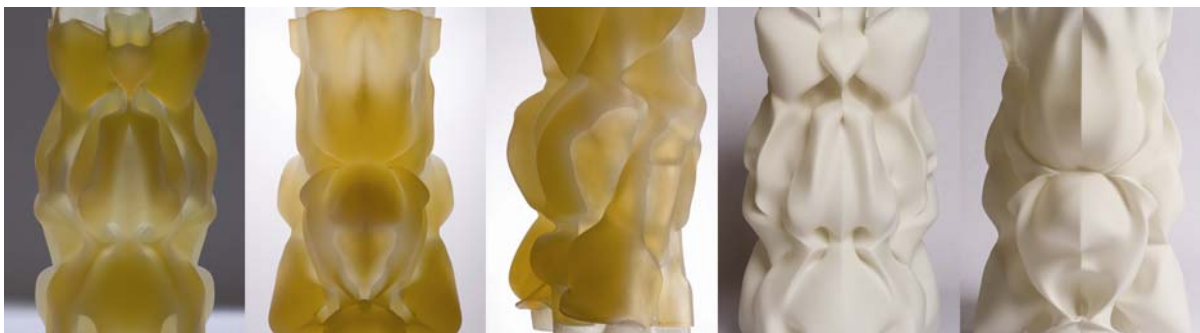
Figure 3. Raycounting: SLS nylon models (top) and printed resin composites including structural pockets (bottom).
